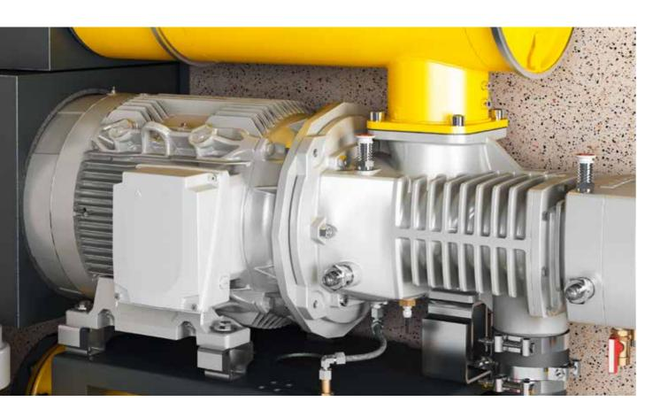
In CBS to GBS series rotary screw blowers, power is transferred from the motor to the blower airend via a loss-less and maintenance-free gear transmission. This has proven to be the best solution for the prevailing speeds in this performance and size class when it comes to efficiency, reliability and durability.
